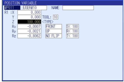
3.1.23 If you forward to this position variable it should take you pointer TCP above the feature you put the cross hairs on. You can move Z- and the pointer should touch that spot. If not go back and complete the calibration again checking pointer TCP and the calibration UF. If it does move to the next step.
